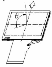
Note 8. The viewing angles are measured at the center area of the panel when all the input terminals of LCD panel are electrically opened.
