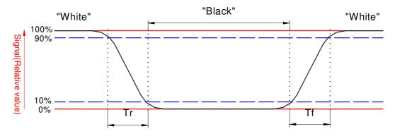
Note 4. From liquid crystal characteristics, response time will become slower and the color of panel will become darker when ambient temperature is below 25°C.
